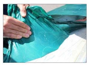
Cortec® VpCI® removable coatings are an excellent option for short- or intermediate-term corrosion protection on valuable equipment and components. They typically leave a translucent, waxy coating that cures to a soft film and eventually hardens. Variations include a thin-film water-based coating that dries clear, a heavy-duty coating for harsh outdoor applications such as offshore layup, and a peelable
