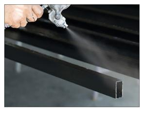
A good primer provides an important baseline for any coatings system, especially when corrosion protection is at stake. Primers provide good adhesion between the metal and topcoat for a stronger barrier against corrosion. They also cover imperfections in the substrate, resulting in a better finish and appearance for the coated equipment or structure. Especially important in the case of VpCI® primers is that they bring corrosion inhibitors in contact with the metal substrate.
